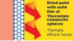
Thermashield contains Thermilate composite spheres which create a thermal barrier. They refract, reflect and dissipate heat.
